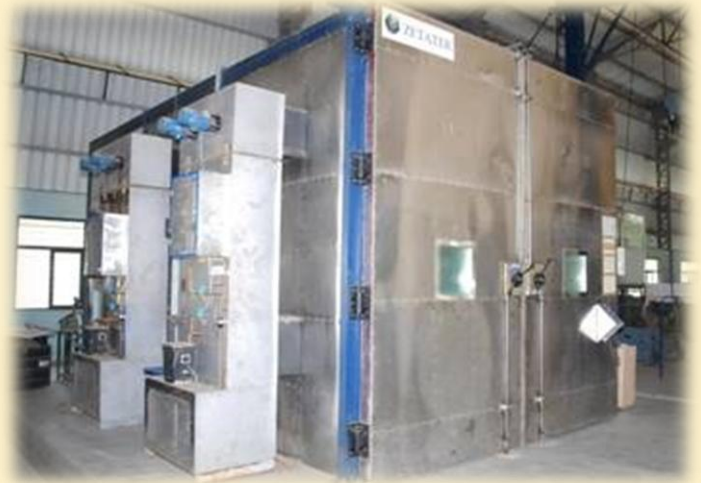
7. Cold Start ability of Engine, Wiping Test System, Demist/Defrost Humid Soak/Corrosion Testing, Climate Ageing Test
